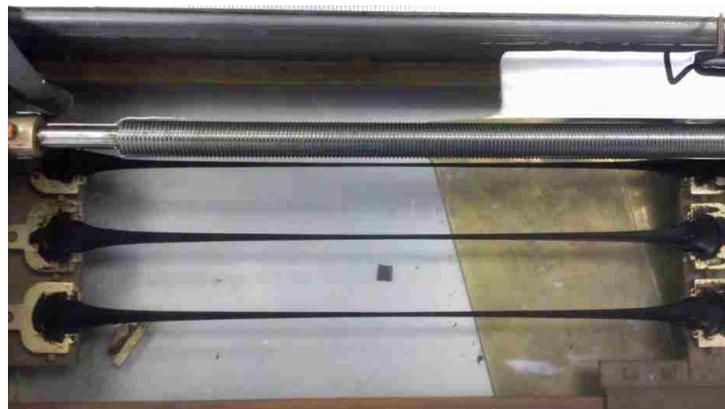
Figure 6-2 Type 1 Failure in the Ductility Test
