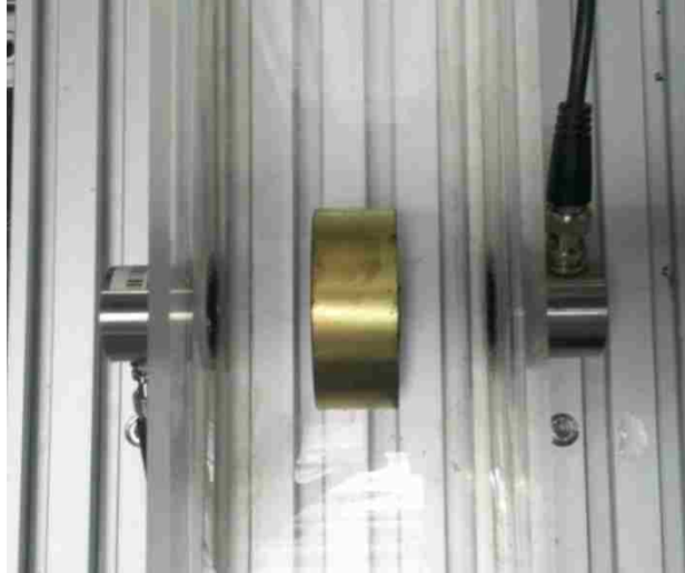
Figure 5-4 Bird's Eye View of the Sample Placed between the Two Transducers
