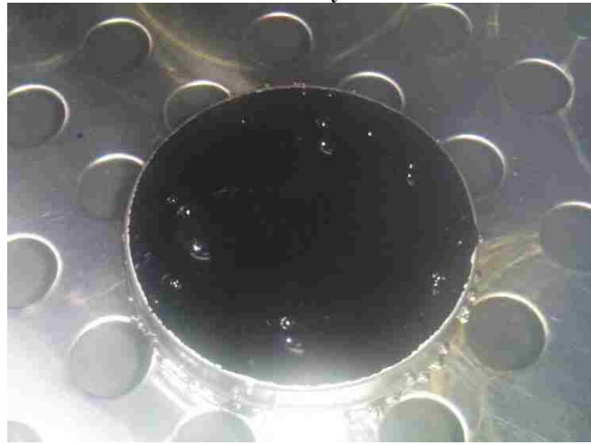
Figure 5-20 Reduction in the Amount of Bubbles after Using Distilled Water
