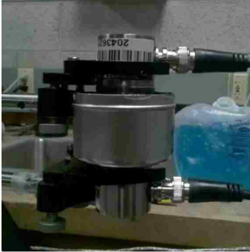
Figure 5-1 Pulse/Receive Contact Measurement Configuration
